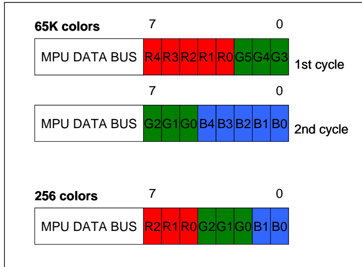
Figure 6-34 : Color illustrations for 8-Bit Data Bus MCU
